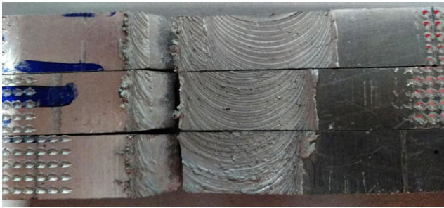
Fig. 15 Fracture localization on the retreating side of the FSP track
