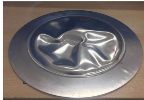
Fig. 1 Photograph of deformed workpiece with wrinkling caused by air resistance
