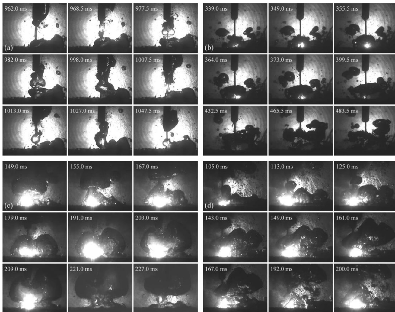
Fig. 11 Comparison of the bubble dynamics under different welding conditions. a At small arc voltage of 22 V without ultrasonic wave. b At small arc voltage of 22 V with ultrasonic wave. c At large arc voltage of 42 V without ultrasonic wave. d At large arc voltage of 42 V with ultrasonic wave
