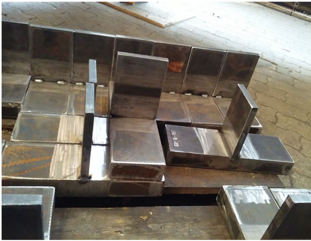
Fig. 1 Tack welded T-joints before welding
