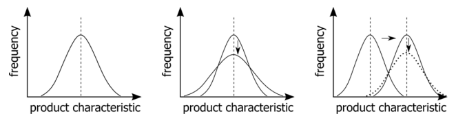
Fig. 10 Effects of existing product characteristics on process results: Product characteristic depends only on probability (left), existing characteristics influence distribution (middle), existing characteristics influence expected value and distribution (right)
