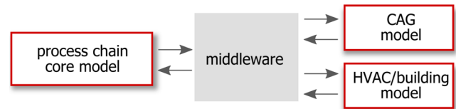
Fig. 13 Model structure for exemplary simulation: A process chain core model is connected with a compressed air generation system model (CAG) and a building model by using a middleware software
