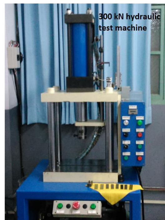
(c) Press for bending experiments
