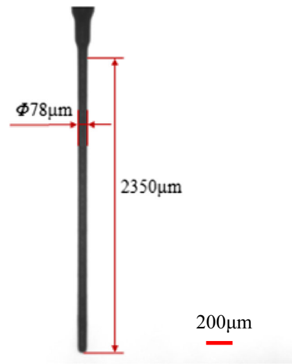
Fig. 4 Micro rod machined by BEDG with spindle rotational speeds of 60,000 rpm
