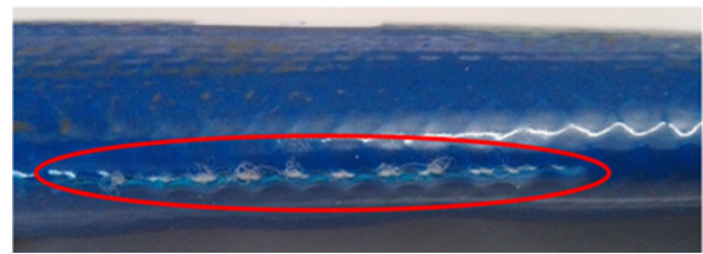
Fig. 16 Failure in hose FTS3
