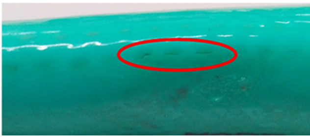
Fig. 17 Failure in hose HFL1
