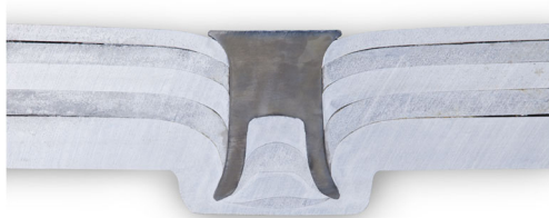
Fig. 25 Cross-sectional shape of the rivet and workpiece plates in multi-layer SPR joining [103]
