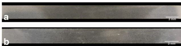
Fig. 3 Cross section macrostructure of processed specimens: a FS and b FSV processed specimens
