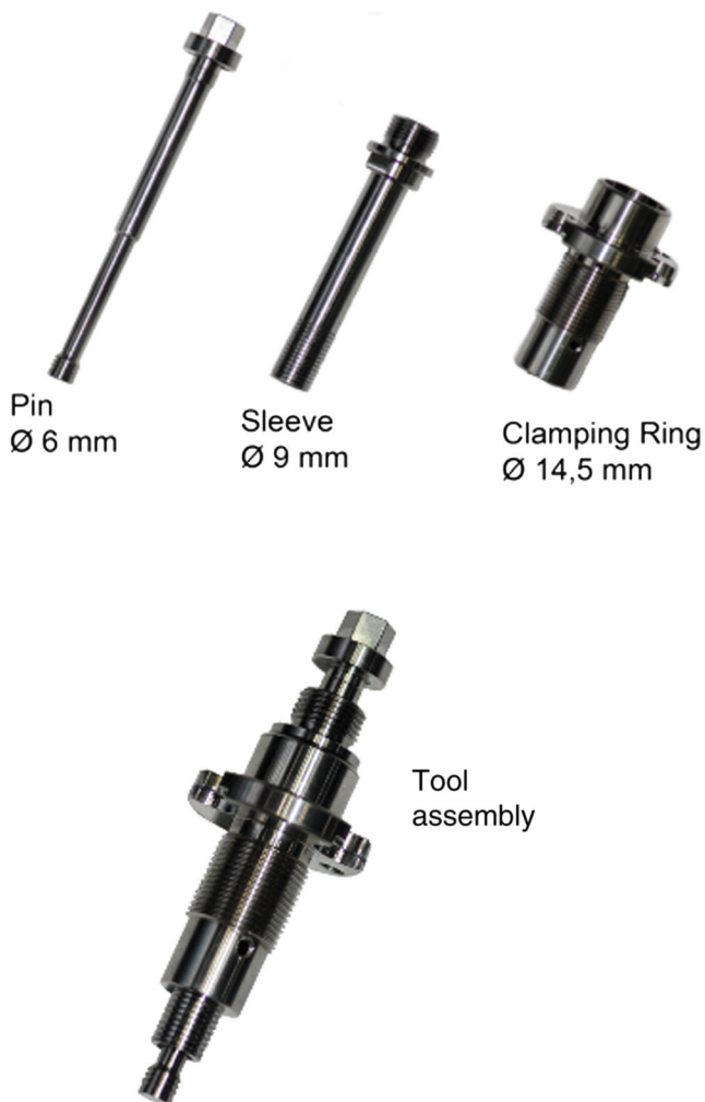
Fig. 1 RFSSW tool: pin, sleeve and clamping ring on the left, and tool assembly
