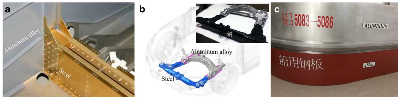
Fig. 1 The typical applications of Al/steel hybrid structures in industries. a Aerospace industry, b automotive industry, and c ship-building industry
