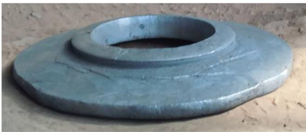
Fig. 6 Shroud disk manufactured by local loading with rotational partial die [43]
