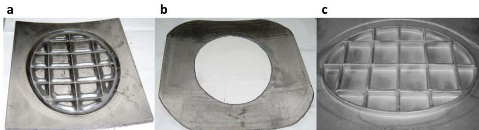
Fig. 4 Aluminum alloy hatch manufactured by local loading method [36]: a transitive die plate, b annular bolster plate, and c forging
