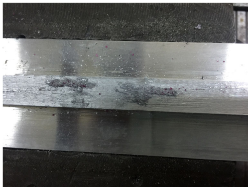
Fig. 5 Photograph of chip adhesion on the workpiece surface
