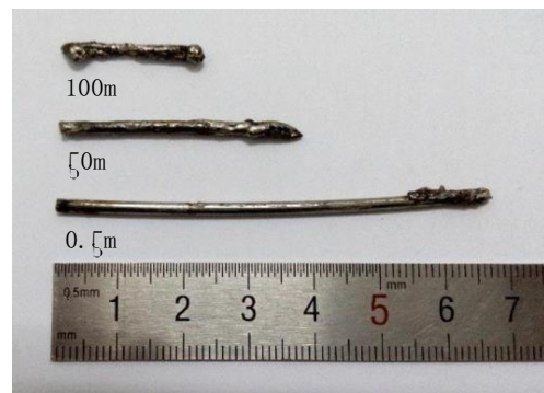
Fig. 11 The average length of broken wire under different water depths
