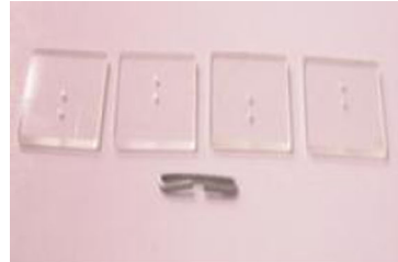
(a) 2mm deep hole drilling in bk7 glass
