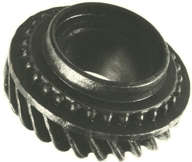
Fig. 17 Helical spur gear with synchro cone and dog teeth forged from a hollow preform in a completely closed die cavity [85]
