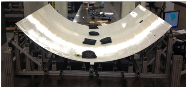
Fig. 2 An aerospace panel under permissible restrained loads (the weight of black sandbags applied on the surface of part) achieves the functional shape on physical fixture [1]
