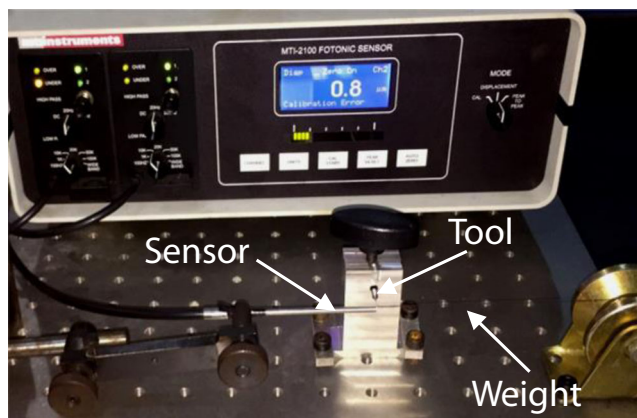
Fig. 4 Measurement for the stiffness of micro-grinding tool
