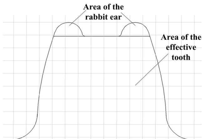
**Fig. 13** The diagram of the tooth area acquired with the mesh tool in Flash software
