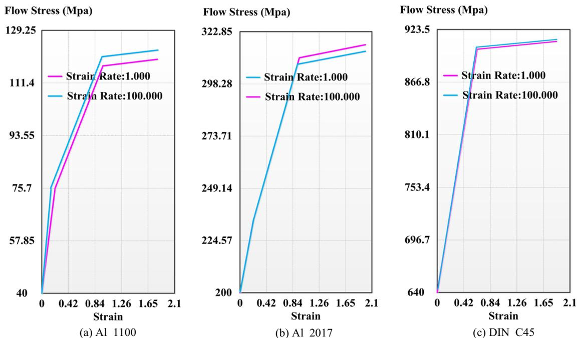
**Fig. 5** Constitutive relationship of three different materials. a Al\_1100. b Al\_2017. c DIN\_C45
