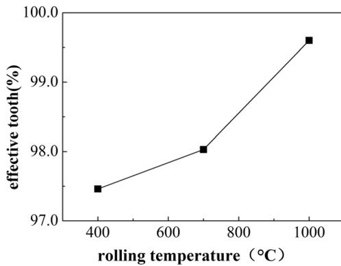
Fig. 9 Changes in the effective tooth volume percentage with different forming temperatures
