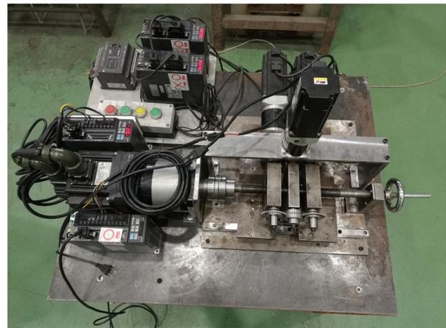
Fig. 11 Gear rolling experimental apparatus
