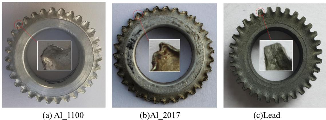
**Fig. 12** The tooth morphology of the specimen with different materials. **a** Al\_1100. **b** Al\_2017. **c** Lead
