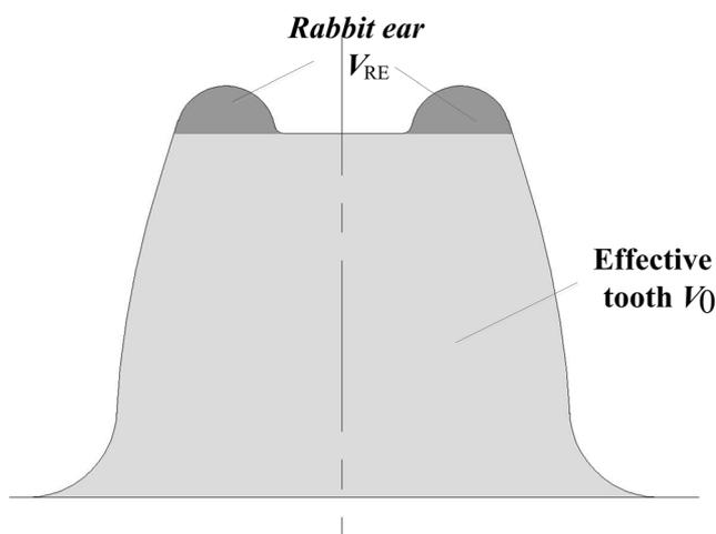
Fig. 3 Volume distribution schematic diagram of the rabbit ear and the effective tooth
