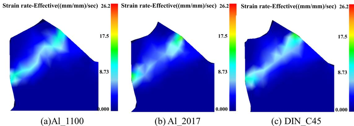
**Fig. 7** Equivalent strain rate of rolled gear with different blank materials. **a** Al\_1100. **b** Al\_2017. **c** DIN\_C45
