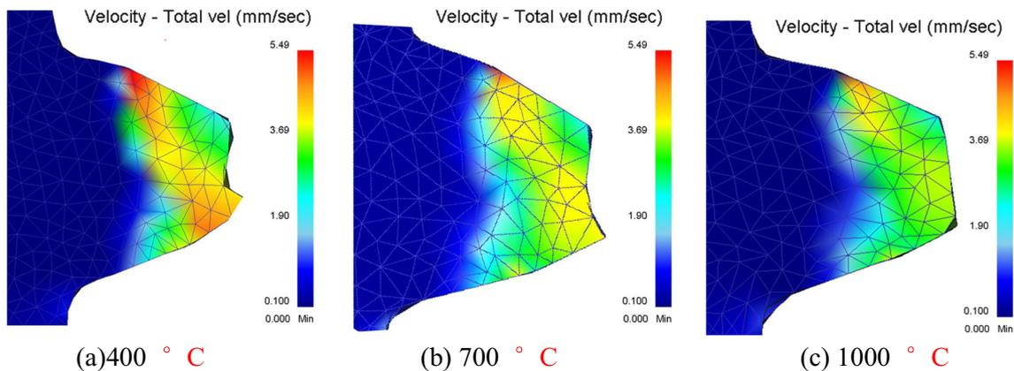
Fig. 10 Isochromatic image of velocity field of the rolled blank in different forming temperatures. a 400 °C. b 700 °C. c 1000 °C
