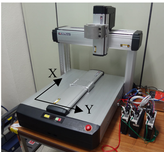
Fig. 3 Two-DOF Cartesian machine used for experiments
