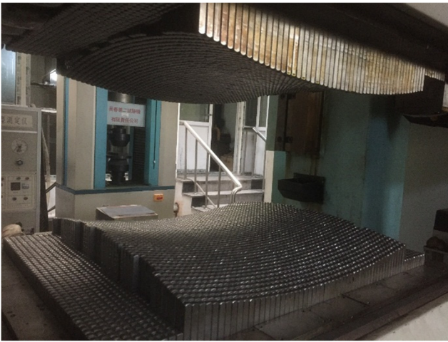
Fig. 1 The work surface of YAM-200 multi-point forming press
