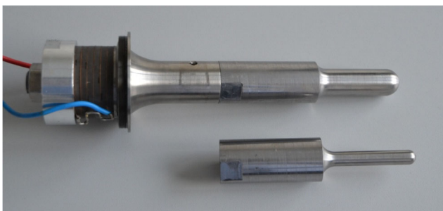
Fig. 2 The transducer and two sonotrodes
