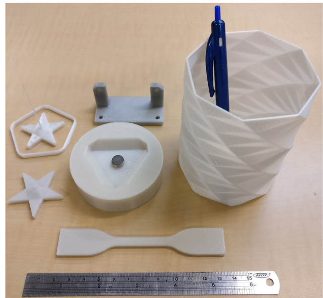
Fig. 8 A variety of printed parts demonstrating the capability of the designed pellet extrusion system
