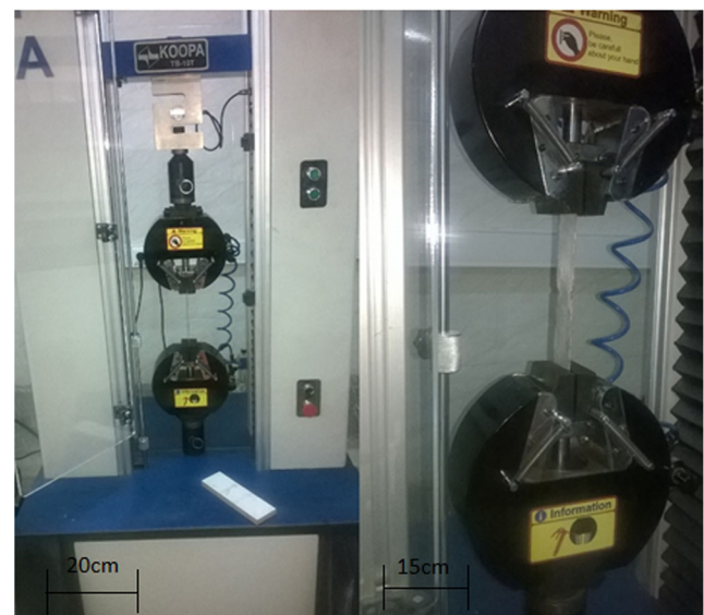
Fig. 10 Uniaxial tensile test on the notched strip sample
