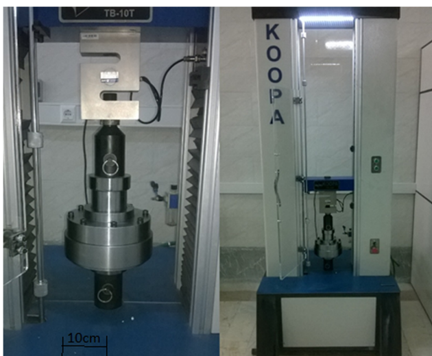
Fig. 9 Stretch forming test with hemispherical punch
