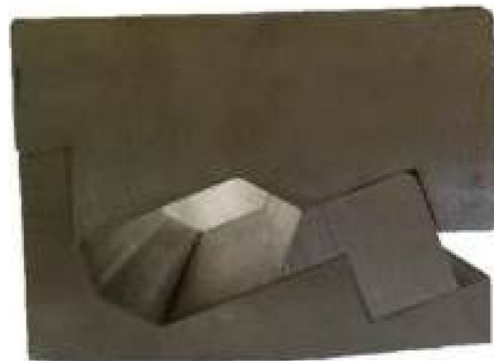
Fig. 3 The three-piece liquid impact forming die
