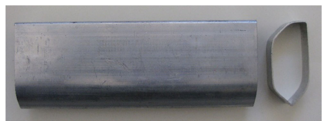
Fig. 12 The test result for tube filled with water at a pressure of 7 MPa
