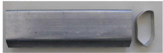
Fig. 11 The test result for the tube filled with water at a pressure of 6 MPa using the three-piece die
