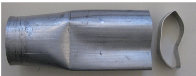
Fig. 10 The test result for empty tube using the three-piece die
