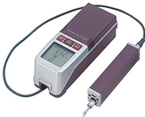
Fig. 3 SJ-201 Mitutoyo device [1]
