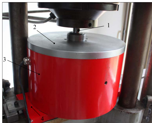
Fig. 2 External profile of the EBHD. (1) Punch. (2) Magnetic plate. (3) Magnetic frame. (4) Baseboard of the device
