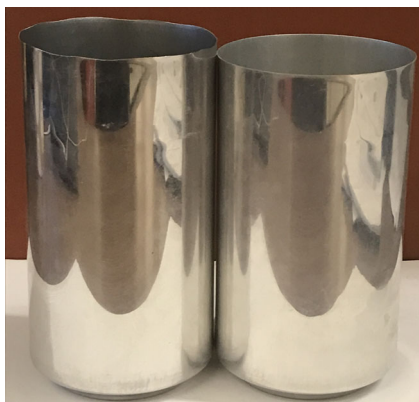
Fig. 2 Experimental samples of untrimmed and trimmed can bodies
