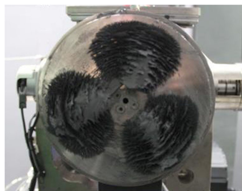
Fig. 10 MR fluid ribbons on polishing lap
