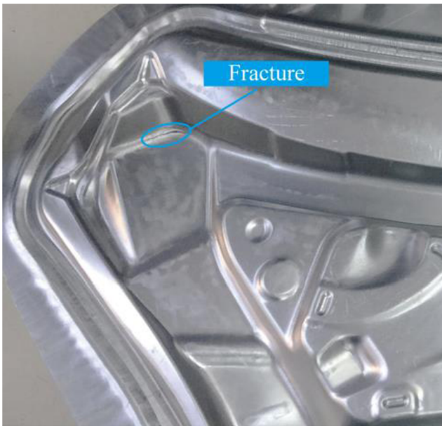
Fig. 17 Fracture at position B caused by hydraulic pressure 20 MPa
