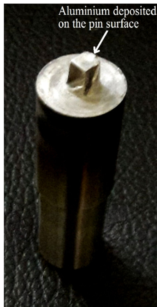
Fig. 2 Tapered FSW square pin profile tool
