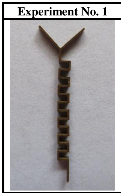
Fig. 3 WED machined square profile copper micro-tool
