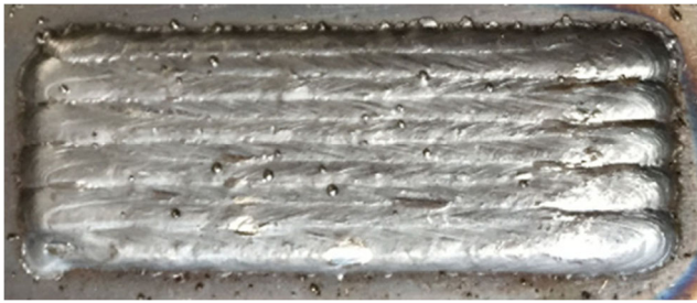
Fig. 25 Fewest joint strategy applied in the plate deposition
