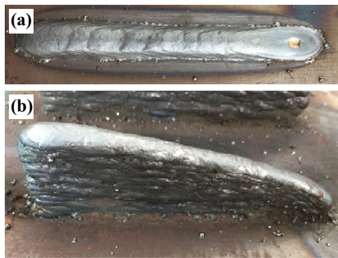
Fig. 1 a Single weld bead. b Thin-walled part with 16 layers single-pass deposited in the same direction (zig)
