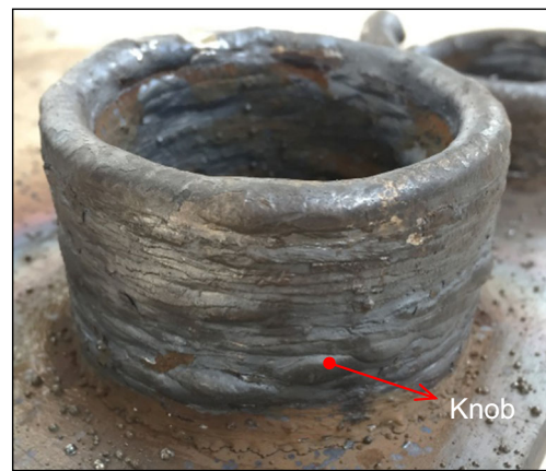
Fig. 21 A cup-shaped component deposited along the same direction with the overlapping strategy
