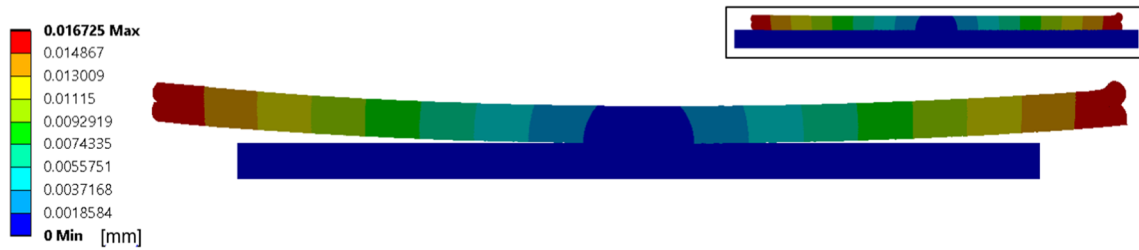
Fig. 9 Warpage exhibited by PPS in the process simulation model. PPS roads 1 and 2 exhibit a warpage of 0.017 mm after cooling together for 10 s. The inset shows the geometry to scale while the main figure is scaled by a factor of 10 to show the shape the warpage exhibits
