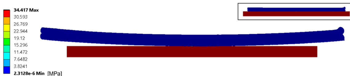
Fig. 10 Residual stresses in roads 1 and 2 at steady state. PPS roads 1 and 2 exhibit minimal residual stress after cooling. The inset shows the geometry to scale while the main figure is scaled by a factor of 10 to show the shape the warpage exhibits
