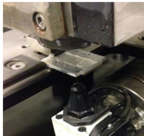
Fig. 5 Cut of traction specimens by wire electrodes. Source: author
