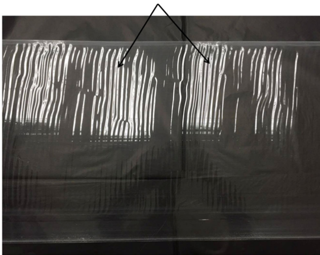
Fig. 6 Wavelike and sharkskin defects on the fabricated polymer film
