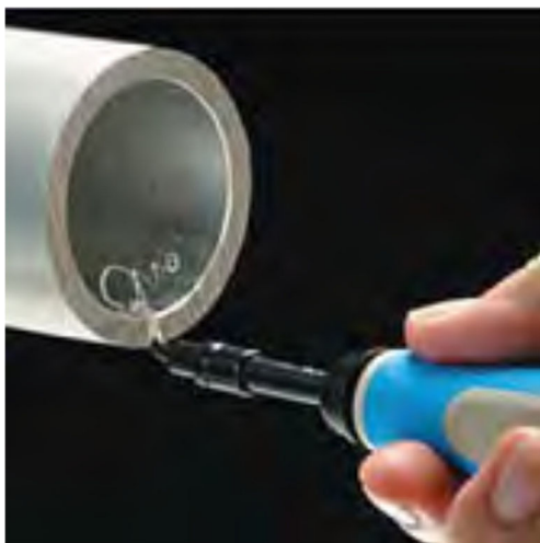
Fig. 9 Manual deburring (Adapted from [98])
