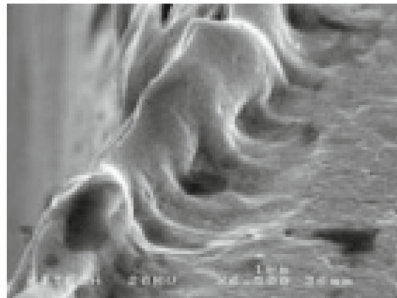
(b) After ultrasonic deburring during 30 sec
