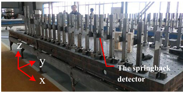
Fig. 11 The springback detector for FSB process
