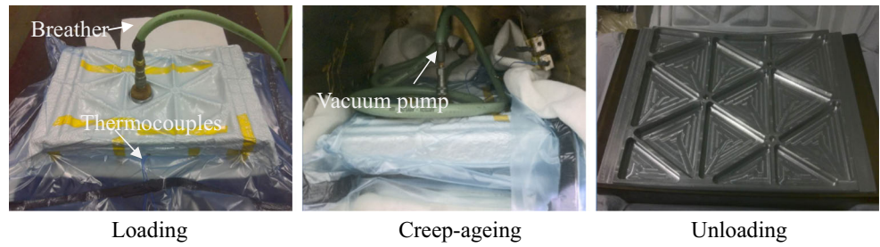
Fig. 5 Creep-age forming of the stiffened plate
