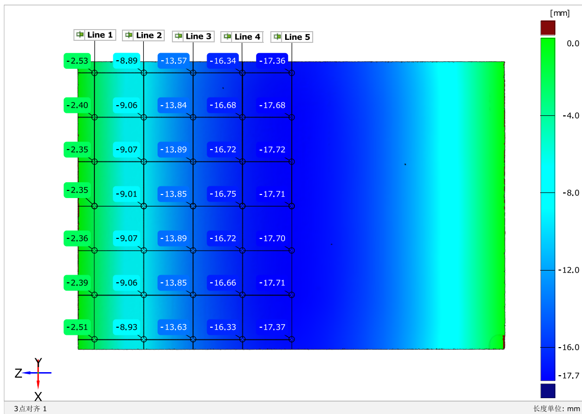
Fig. 15 Deflection distribution between outer surface of the formed plate and initial flat plate
