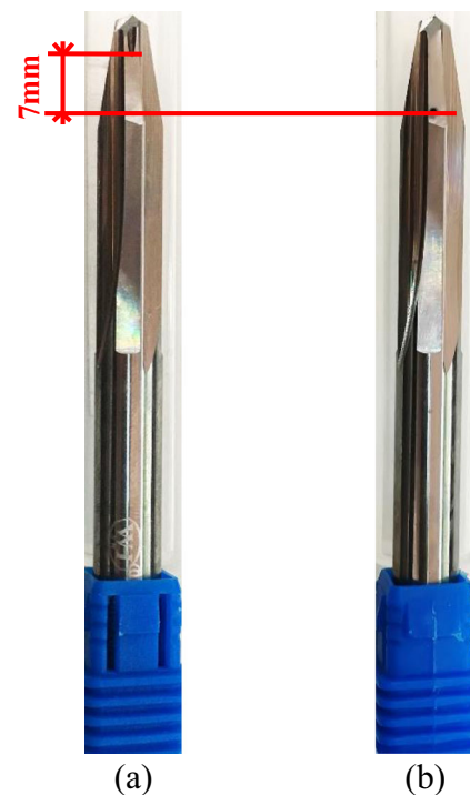
Fig. 1 One-shot drill bits with different MQL supply outlet positions (a) #1 drill bit, MQL outlets located at the front of the secondary cutting edges, (b) #2 drill bit, MQL outlets located at the end of the secondary cutting edges
