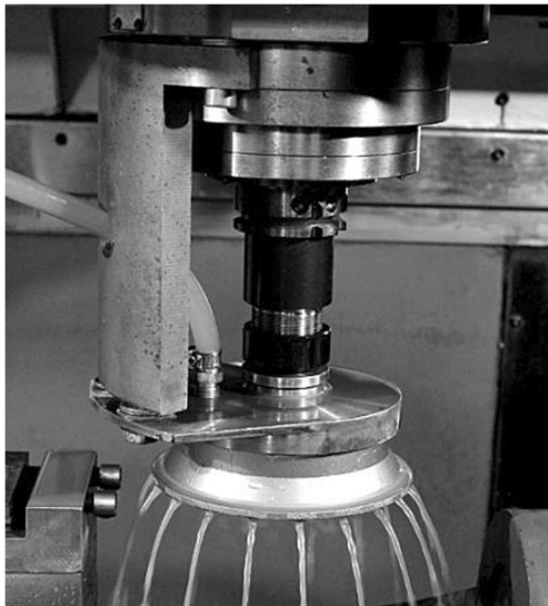
Fig. 21 Grinding wheel system with coolant supply
