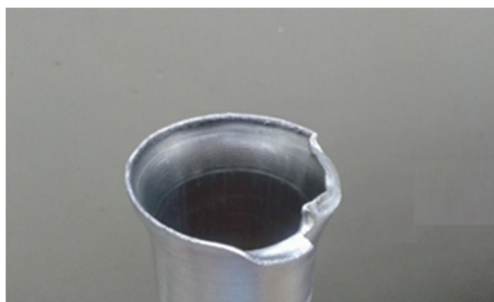
Fig. 7 A failure in incremental tube end flaring due to an improper positioning of the forming tool at the second stage
