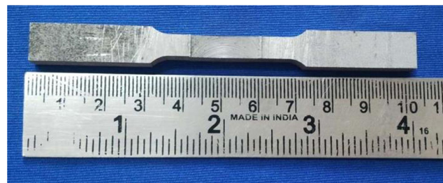
Fig. 4 Tensile sample of the friction stir welded joint
