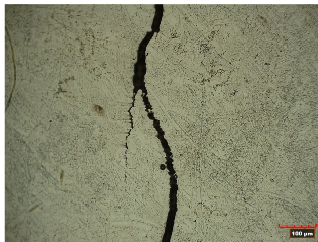
Fig. 11 Optical image of a transverse cross-sectioned laser deposit showing a crack
