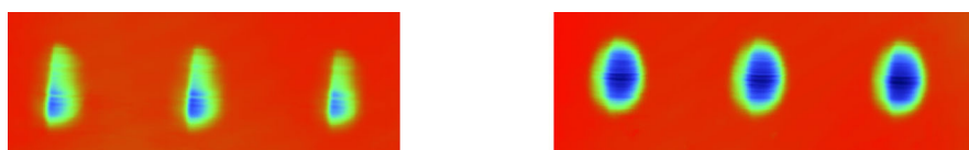
(a) spots polished by severe worn tool surface (b) spots polished by conditioned tool surface
