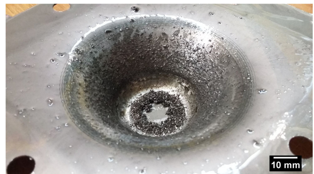
Fig. 13 Scratched sheet, heat-treated, formed by hemispherical head tool rotating
