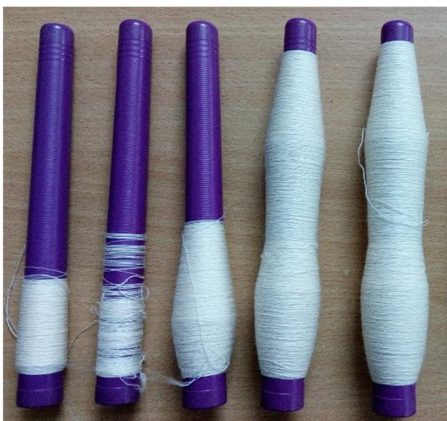
Fig. 4 Defective ring cops
