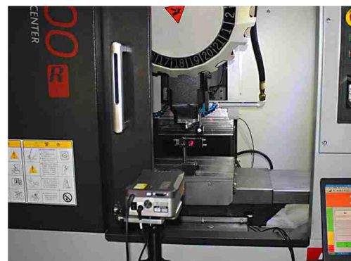
Fig. 5 Test of thermal errors using a laser interferometer
