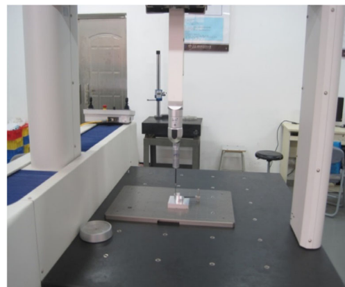
Fig. 8 The detecting scene of coordinate measuring machine
